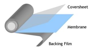
The backing film facilitates transporting the membrane into automated MEA fabrication processes, while the coversheet protects the membrane from exposure to the environment during intermediate handling and processing. In addition, the coversheet (in combination with the backing film) eliminates rapid changes in the membrane's moisture content, and stabilizes the dimensions of the membrane when removed from the roll.
